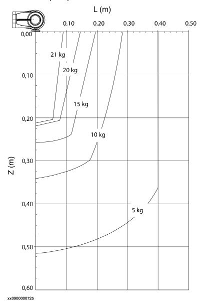
Extra load of 10 kg at the upper arm housing and 1 kg at wrist included in the load diagram.
