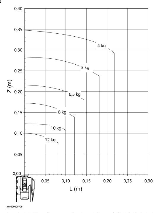
Extra load of 10 kg at the upper arm housing and 1 kg at wrist included in the load diagram.
